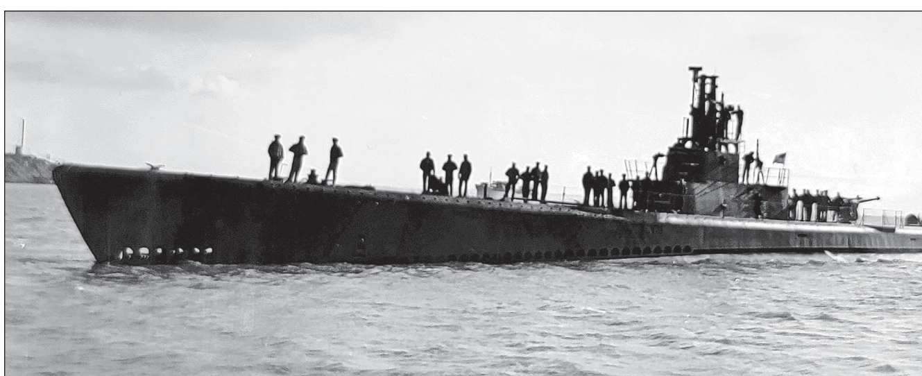
These photos of Albacore, taken two years apart, show the extent of the modifications it underwent during its brief life. Like other Gato-class subs, it had a large conning tower fairwater, the structure amidships, which was seen as a liability in combat. Gatos underwent three modifications to reduce their profile. The top view was taken at Electric Boat on May 9, 1942. Below is how Albacore looked at Mare Island Naval Shipyard after the third modification on April 28, 1944.
